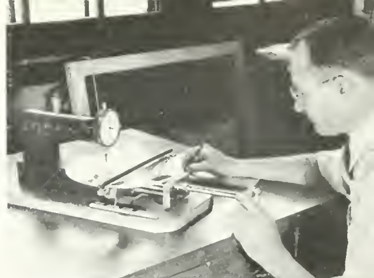
R. LEUSCHNER TESTS AN ASPHERICAL LENS (ABOVE) FOR DEVIATIONS FROM THEORETICAL DESIGN; THE AUTHOR REMOVES A PLASTIC ASPHERICAL LENS (BELOW) FROM THE MOLD IN WHICH IT WAS MADE.
