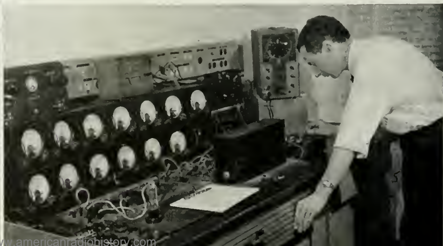
LIQUID AIR, TEMPERATURE 313 DEGREES BELOW ZERO, FAHRENHEIT, IS USED BY J. BURNETT TO IMPROVE THE VACUUM IN A TUBE WHEN IT IS COMPLETED. BELOW, H. A. FINKE TAKES PERFORMANCE DATA ON A BEREARCH TUBE AS IT IS PUT THROUGH ITS PACES IN AN ELABORATE SERIES OF ELECTRICAL TESTS.
